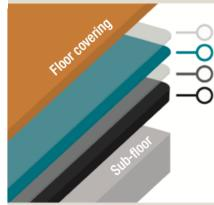
Protective Release Film Adhesive Membrane Non-Woven Polypropylene Scrim Recycled Rubber Crumb
